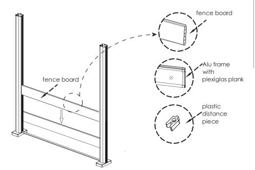
4-1.A is the shown drawing for fence board with distance pieces, B is the shown drawing with Alu Frame with plexiglas plank.
