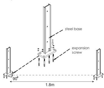
2.Make sure to put Steel Base Cap firstly. Use two screws to connect the Steel Base and the ALU Post.
