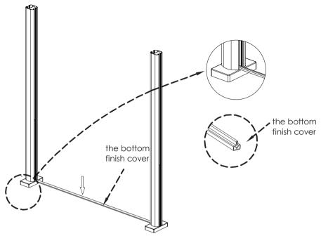
4.Slide the fence board along the WPC post grooves one by one, these fence boards linked together and form a wall.(refer to 4-1
