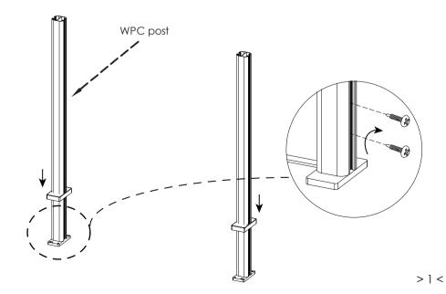
3.Slide down the bottom finish cover along the WPC post grooves to the bottom.
